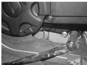
The Engine number is stamped on the left bottom side below the crankcase. Also
