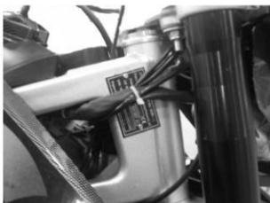
The VIN plate is located on the top right side of the frame and the VIN is stamped on the head of frame.
